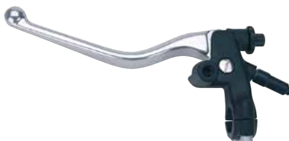
COD. 2609.04 Mod Custom Sinistro con leva lucida Left with polished lever fulcro leva - lever fulcrum mm 30 per - for Betamoto Euro - Jonathan Gilera Coguar
