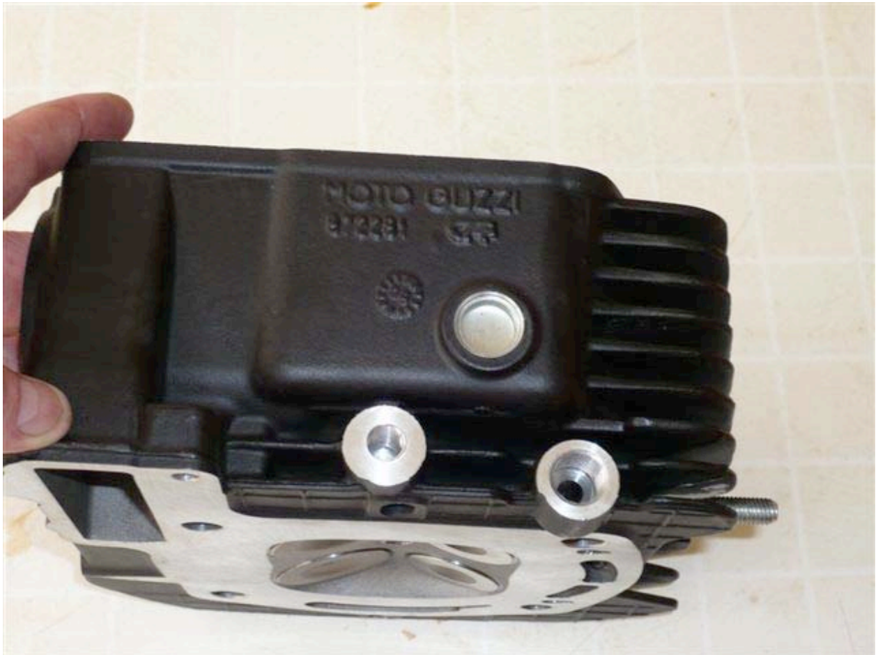
Looking at the valley side of the head you can see the lubrication oil feed. That is the hole at the front of the head in line with the exhaust stud. This feeds oil into the upper forward stud hole.
