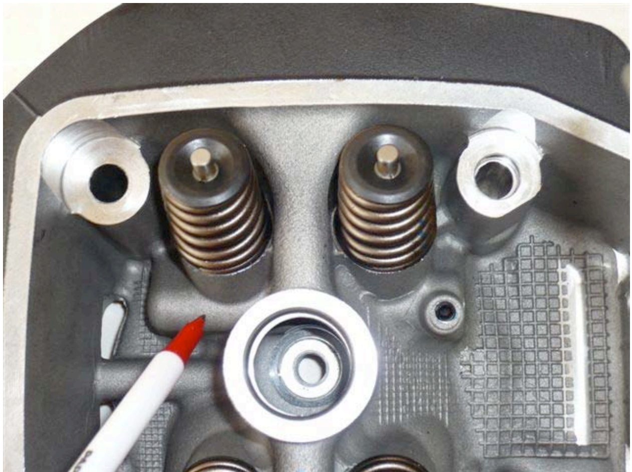
You can see here the boss the gallery is drilled through in the casting.
