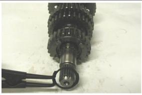
• Remove the gear of the sixth gear.
