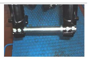
• Tighten the screws on the fork plates to the prescribed torque.
