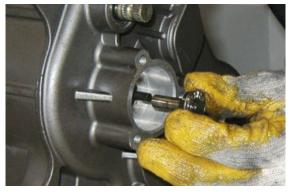
Slide off the rod with the two bushings.
