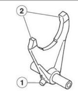
Check the transmission fork movement and if it is not regular, replace the transmission forks.
