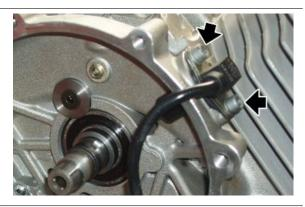
Insert a suitable plain washer on the sensor and note its thickness.
