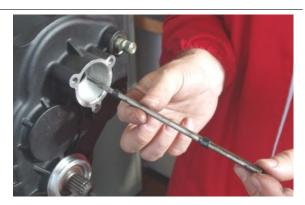
Undo and remove the five external screws.
