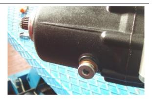
Place a container of suitable capacity under it, unscrew and remove the cap and then bleed all gearbox oil.
