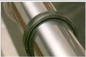
Fit the ring, the movable bushing and, after removing the tape, fit the fixed bushing.
