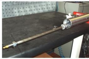
Tighten the screw fixing the pumping member on the fork end to the prescribed torque.
