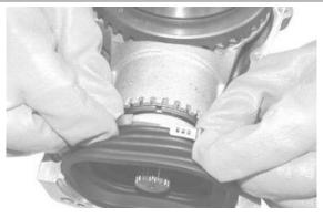
Screw the clamp with the specific pliers.
