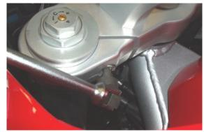
Unscrew and remove the fork upper plate cover; collect the shim.
