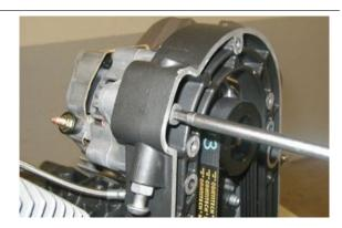
Position the screw and tighten the nut.
