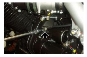
Disconnect the starter motor connectors.
