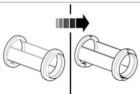
Fit the sleeve on the stem and with the specified tool fit the oil seal into position.
