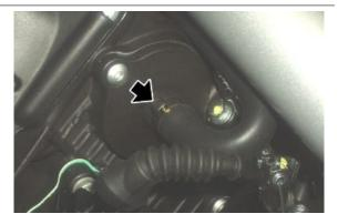
Working on both sides disconnect the injector connectors.
