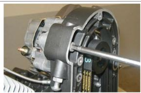
Remove the belt and the alternator with pulley.
