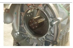
Collect the shim washer from inside the crankcase.
