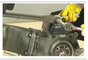
Undo and remove the four screws.
