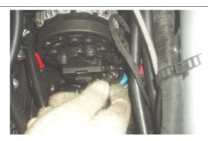
Disconnect the engine oil pressure sensor connector.
