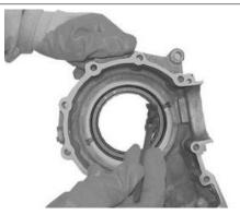
Assemble two centring stud bolts with M8 thread in the threaded holes of the casing as shown in the picture.
