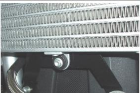
Undo and remove the two radiator upper screws and collect the washer.
