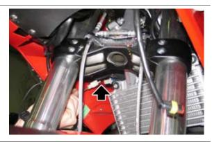
Slide off the cables from the opening near the arrows between the side fairings and fairings.
