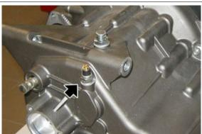
From the outside, slide off the thrust cylinder and collect the O-Ring and the washer.
