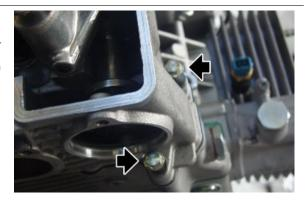
Using a thin screwdriver relief oil pressure from the left cylinder chain tensioner.
