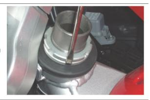
Using the suitable special tool, unscrew and remove the upper ring nut.
