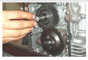
Insert the joint in the oil pump.
