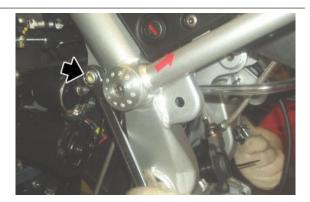
Working on both sides, insert the washer and screw the screw without tighten it.
