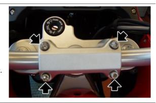
Working on both sides, unscrew and remove the upper plate fixing screw on the fork stems.
