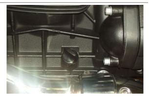
Undo and remove the fourteen screws fixing the oil sump to the engine crankcase.
