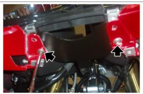
Operating from both sides, disconnect the turn indicator connector.
