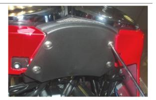
• Unscrew and remove the two screws.
