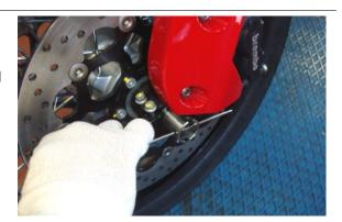
Collect the spacer from the front wheel right side.
