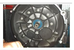
Open the gearbox using the specific tool.
