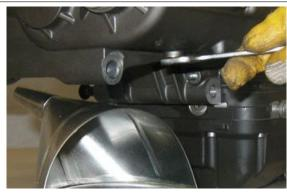
Loosen and turn the oil pipe fitting on the sump.
