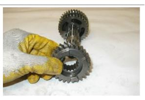
• Remove the circlip and collect the shoulder washer.
