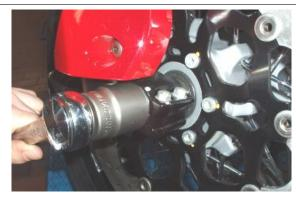
Working from both sides, loosen the screws on the wheel bolt clamps.
