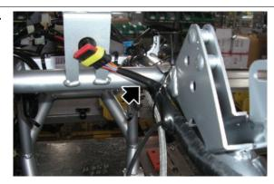
The connection must be between the chassis and the air filter.
