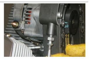
Completely loosen and remove the screw.
