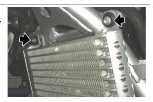
Undo and remove the radiator lower screw and collect the washer.
