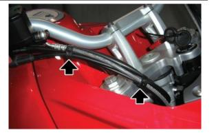
Clamp the clutch pipes with the clutch switch and the left light switch, making sure that the fixing part of the lower clamp faces the inside, to avoid that by turning the steering the instrument panel is damaged and the clamp gets unhooked.
