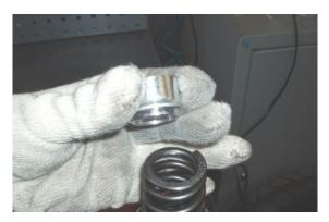
Remove the spring. Let the oil deposited on the spring turns fully drip into the sleeve.
