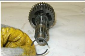
Remove the gear of the fifth gear and collect the ball bearing cage.
