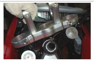
Rivet the safety washer on the headstock.
