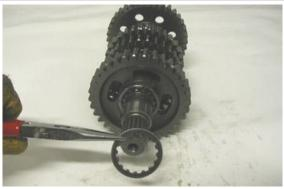
Remove the gear of the second gear and collect the ball bearing cage and the shoulder washer.
