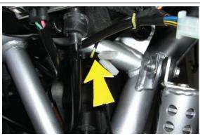
Pass the cable harness under the beam.
