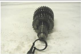
• Remove the gear of the third and fourth gears.
