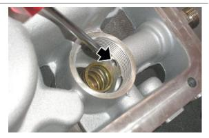
• Tighten the thermostatic valve plug.
