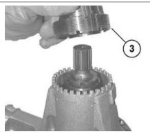
Assemble the sealing ring (3) to the ring nut (2) with the buffer CA715855 (see Fig.1) and a hammer.
