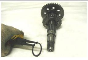
• Remove the gear of the fifth gear.
