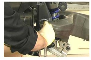
Helped by a second operator, remove the pin and remove the swingarm together with the cardan shaft.
