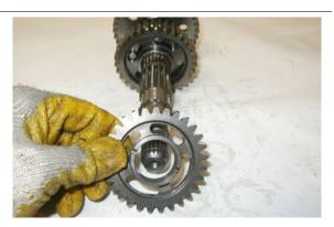
Remove the gear of the third gear and collect the ball bearing cage and the shoulder washer.
