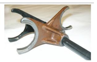
• Remove the forks and collect the shaft.
