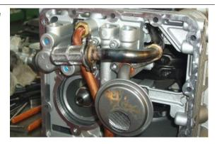
Fix both filters and tighten the two screws to the prescribed torque.
