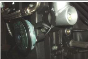
Operating from both sides, undo and remove the screw fixing the oil radiator to the chassis.
