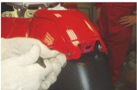
Unscrew and remove the front screw fixing the tank.
