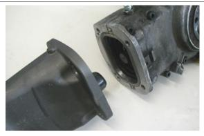
• Tighten the four screws to the prescribed torque operating diagonally.
