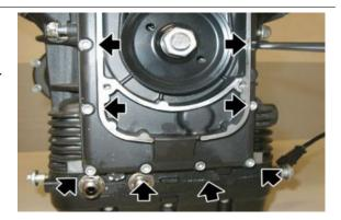
Tighten the four screws, operating diagonally and in stages.
