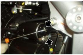
Disconnect the stand sensor connector and release it from the clamps.
