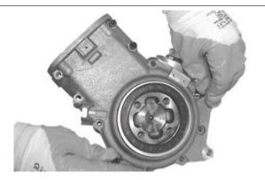
Assemble the ring to the casing.
