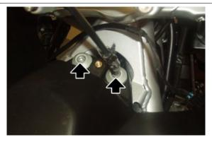
Lift the tank and disconnect the fuel pipe.
