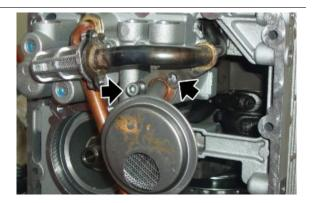
Unscrew and remove the plug.
