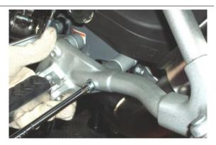
Undo and remove the lower screw and collect the washer and the spacer.
