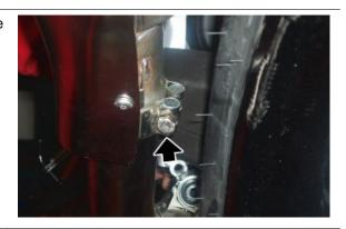
Undo and remove the screw and collect the nut and the washer.
