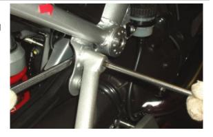
Undo and remove the front lower screw.
