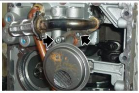
• Fit a new oil filter and tighten it to the prescribed torque.
