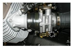
Remove the two breather pipes.
