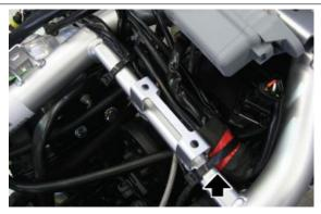
The cable of heated handgrips must come out under the beam and be clamped.
