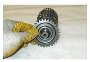
Remove the circlip.
