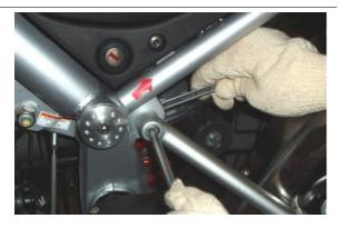
Undo and remove the lower screw and collect the two washers and the spacer.
