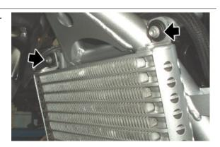
Remove the oil cooling radiator.
