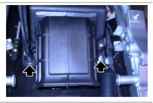
Disconnect the air temperature sensor connector.
