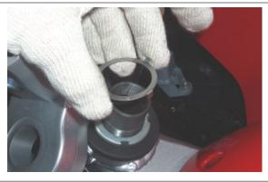
Using the suitable special tool, set the preloading of the steering bearings.
