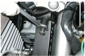
Tighten the alternator fixing screws.
