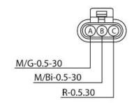
THE CONNECTION DIAGRAMS ARE IN THE ELECTRICAL SYSTEM SECTIONS; PAY ATTENTION TO THESE DIAGRAMS AS THEY SHOW THE CONNECTOR/COMPONENT AS VIEWED FROM THE CABLE HARNESS SIDE, THAT IS LOOKING AT THE CABLES WHEN GOING OUT OF THE "MAIN" CABLE HARNESS AND INTO THE CONNECTOR/COMPONENT.
