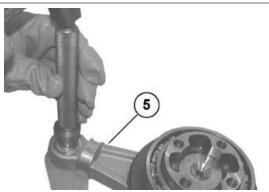
Fit the stop ring (3) in the support (5) with suitable pliers.
