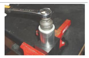
Push the bushing down in order to compress the spring and then fit a tool under the pumping member lock nut and on the bushing to keep the spring compressed.
