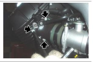
Connect the stand sensor connector and fix it to the chassis with new clamps.
