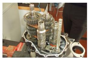
Remove the bearings from the gearbox if necessary.
