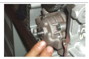
• Place the gear on the oil pump shaft.
