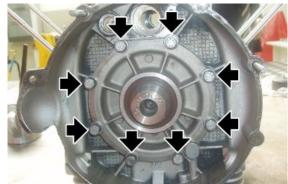
Remove the sealing ring centring tool from the crankshaft.
