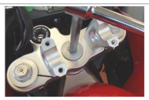
Lift the fork upper plate sliding it off from the stems.
