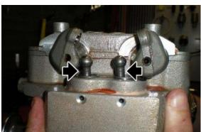
Place the two rocking levers in the cam tower seats.
