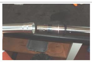
From the stem remove the fixed fitted bushing, the movable bushing, the ring and the oil seal.
