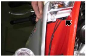
Remove the screw (M8x20) and be careful to collect the washer and the nut.
