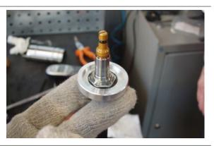
Insert the preloading pipe with the two spring guides in the sleeve.
