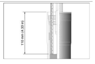
Measure the air gap between the oil level and the rim.
