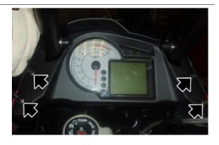
Disconnect the instrument panel connector.
