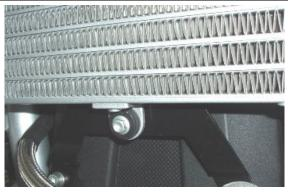
Undo and remove the horn fixing screw.
