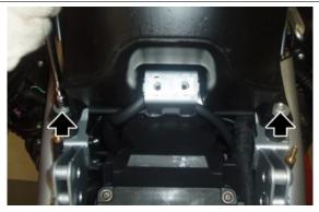
Undo and remove the two front screws.
