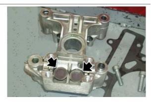
Place the camshaft with the gear seat on the dowel side.
