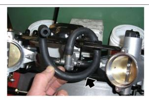
The shortest part of the fuel pipe connected to the throttle bodies should be placed on the right.
