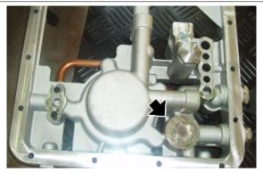
• Remove the thermostatic valve.
