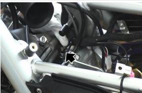
Connect the alternator connectors.
