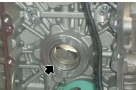
• Use the sealing ring fitting tool on the flywheel-side flange to fit the sealing ring on the flange.
