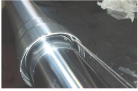
Fit the dust guard with the specific tool.
