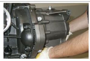
Unscrew and slide off the odometer gear and collect the abutment washer that is inside the gearbox.
