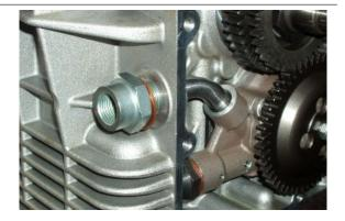
• Remove the nipple - oil pump fitting.
