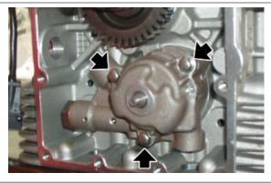
Place the driving pin on the oil pump shaft.
