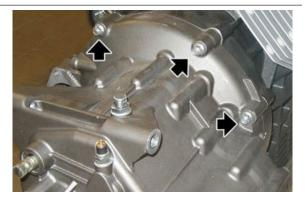
• Undo and remove the two screws.
