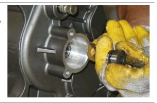
Remove the thrust bearing and the washer.
