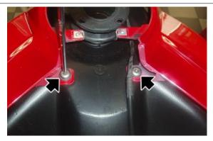
Operating from both sides, undo and remove the internal screw and collect the washer and the nut.
