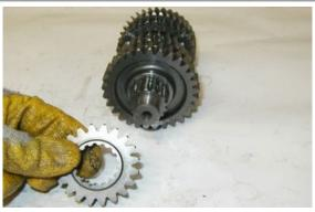
Remove the gear of the sixth gear and collect the shoulder washer.
