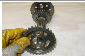
• Remove the circlip.
