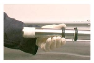
The sealing ring must be placed with the stamped part facing the dust gaiter.
