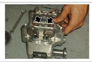
Remove the two rocking levers from the cam cap.
