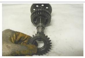
Remove the circlip and collect the shoulder washer.
