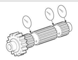
Check transmission gears for signs of pitting and wear and replace damaged gears if necessary.
