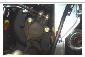
• Connect the starter motor connectors.
