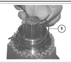
Unscrew the ring nut (2) with the special spanner (s4).
