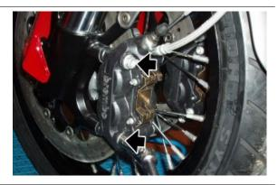
Turn the pins and remove both split pins.
