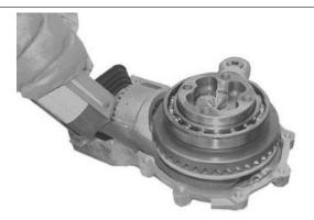
Fit a new sealing ring using the buffer.
