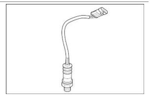
Closed loop indicates that the control unit is using the lambda probe signal to keep the combustion as close as possible to the stoichiometric value.
