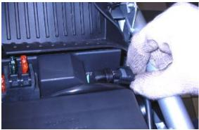
Slide off and remove the main fuse box from its holder.
