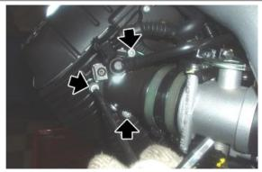
Disconnect the alternator connectors.
