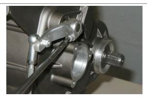
Unscrew and remove the gearbox oil filler cap.
