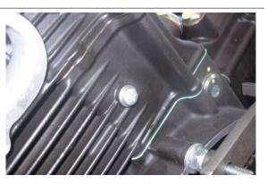
• Check that the oil in the left cylinder chain tensioner has been drained off by compressing it. If the operation is difficult, use a pin drive to push the central hole so that the oil is drained off from the circuit.
