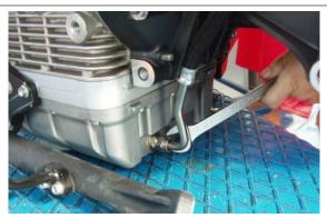
• Undo and remove the three screws.
