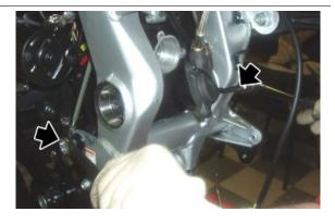
Operating from both sides, tighten the upper engine fixing nut on the internal side of the chassis.
