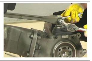
Place the dust-protection ring between the rim and the cardan shaft taking care to mount it with the collar facing the transmission unit.
