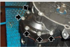
• Place the gearbox on the specific gearbox support tool and on a vice.
