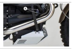
Remove the TCEI screw (9) (M8x60) and the corresponding washer.
