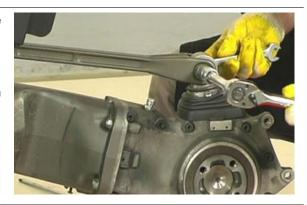
Remove the clamp from the dust guard cap.
