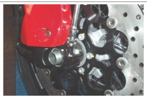
Hit the wheel pin slightly with a rubber hammer so that the hole on the opposite side is exposed.
