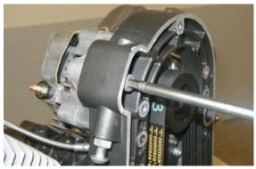
Loosen the nut and undo the set screw so that the alternator slides down.
