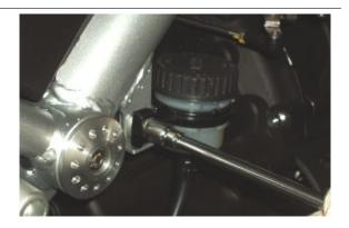
• Remove the right footrest plate, keeping the brake fluid reservoir in vertical position.
