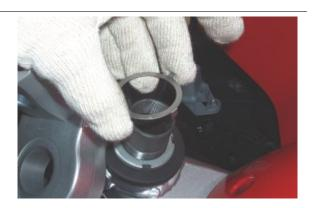
• Screw the upper ring nut manually and then slightly tighten the clamps on the plate so as to align notches on the ring nut.
