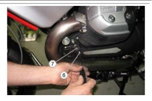
Remove the TCEI screws (8) (M10x35) on the upper side.
