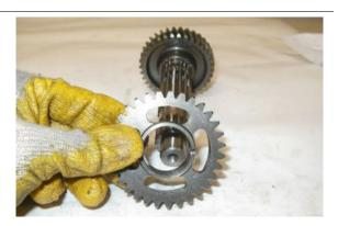
Heat the shaft with a specific heater and remove the helical transmission gear.
