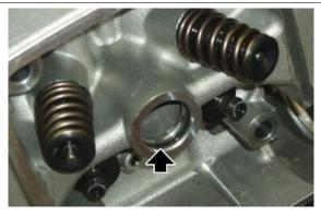
Fix the cam cap with the four nuts on the stud bolts.
