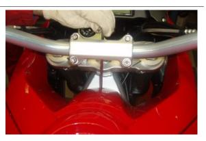
Operating from both sides, undo and remove the two screws.
