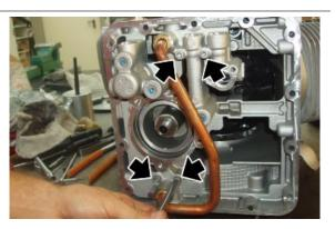
Fit the lubrication oil intake filter.
