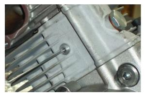
Slide off the timing system gear from the chain to remove it from the camshaft.
