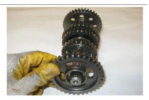
• Remove the circlip.
