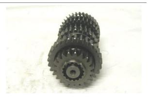
Remove the gear of the second gear and collect the ball bearing cage.
