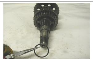
Remove the gear of the fourth gear and collect the ball bearing cage.
