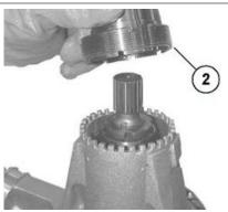
Tighten the ring nut (2) with the special spanner (s4) to the prescribe torque.
