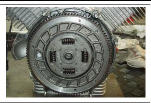
Remove the clutch bell and the friction disc.
