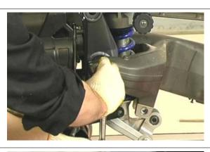
Tighten the two swingarm terminal screws.
