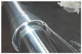
Take out the sleeve from the stem using the stem as a hammer puller.
