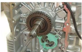
Fit the timing system gear and align the reference with that on the crankshaft gear. Turn the crankshaft to align the two gears.
