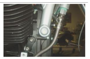
Operating from both sides, undo and remove the upper engine fixing nut on the internal side of the chassis.
