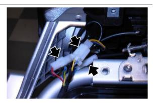
Release the clutch bleeding pipe from the cable guide.
