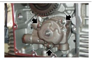
Remove the gasket between the crankcase and the oil pump.
