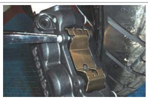
• Remove the vibration-damping plate.
