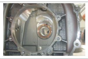
Lubricate the crankshaft bushing on the crankcase, generator side.
