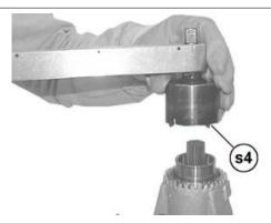
Insert the stop ring (1) in the ring nut (2) in the indicated direction.
