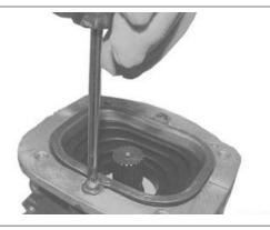
Fit the cap with the washer.
