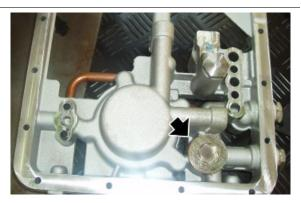
Place a new gasket between the crankcase and the flange.
