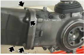
Remove the transmission casing sliding off the universal joint.
