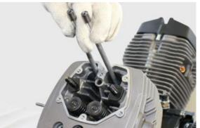
Remove the outer nuts that fix the head to the cylinder and collect the washer
