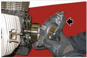
Place the 12 cover fixing screws and tighten them to the prescribed torque
