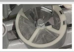
Position the gasket between the sump and crankcase (always change the gasket). Pay attention during the procedure; if wrongly installed, the gasket will prevent proper oil circulation.
