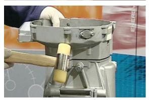
Slacken the lock nut and unscrew the pre-selector positioning eccentric screw.
