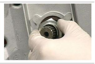
Position the retaining plate and tighten the screws with their washers with threadlocker.
