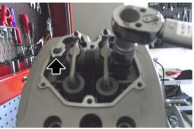
• Tighten the nuts to the prescribed torque following a crisscross pattern.
