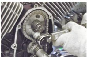
Tighten the oil pump nut while holding the oil pump shaft steady.
