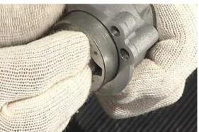
Slide off the bearings and their inner housing from pump body.
