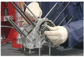
Insert the timing system side and flywheel side half-bearings with their thrust washers into the seats in the upper crankcase.
