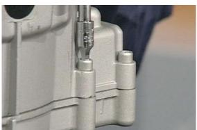
Tighten the clutch shaft nut using the suitable tool and squash.
