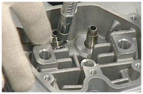
Valve guides need to be knocked out tapping from the inside with punch and mallet; heat the head up to approximately 50-60 °C to aid removal.
