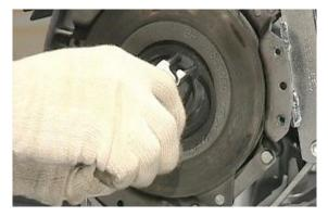
Position the specified clutch plate centring tool on the plate and fit the plate into place.
