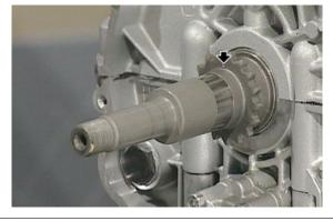
Place the camshaft with the reference pin of the gear pointing downwards.
