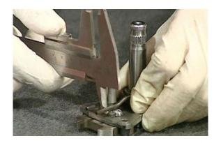
Refit the eccentric screw to the cover together with its lock nut and make sure that the eccentric end of the screw is facing the selector nut.
