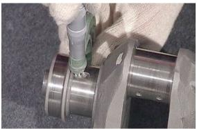
The maximum parallelism deviation of the two crankshaft axes (connecting rod pin and main journals on flywheel side and timing system side) should not exceed 0.02 mm (0.0009 in) at 40 mm (1.5748 in) distance.
