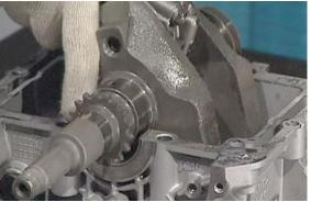
Unscrew the oil pressure sensor from the upper crankcase and remove the retaining bushing of the camshaft; remove the shaft and the tappets, noting their positions.
