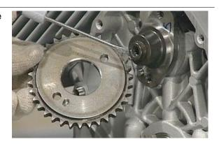
• Insert the oil pump shaft (pin) key.
