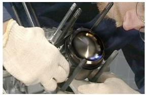
When finished, remove the tool and insert the second snap ring that closes the piston pin seat, after protecting the cylinder seat.
