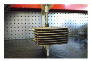
Close the tool to compress the spring, and then hit the tool head with a mallet so that the two cotters get detached from the upper cap.
