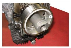
Tighten the threaded pin (2) of the tool and proceed with the rotor removal.
