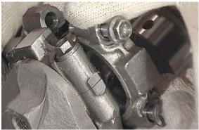
Remove the half-bearings from connecting rods and small ends.
