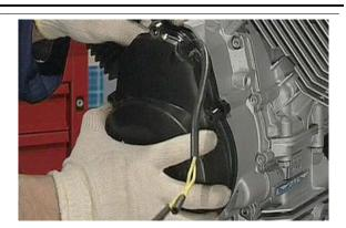
Tighten the five cover fixing screws to the prescribed torque.
