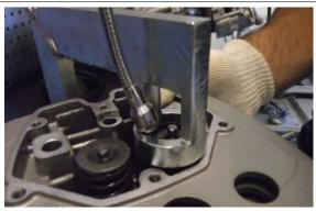
Unscrew the tool and remove it from the head.
