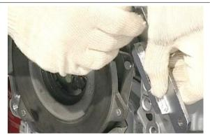
Tighten the screws following a crisscross pattern with a torque wrench set to the prescribed torque. It is advisable to change the fixing screws securing flywheel to crankshaft.
