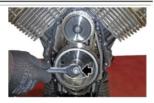
Insert in the rotor hole the specific spacer
