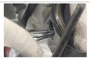
Slide off the pin using the specified tool (turn the tool screw) and remove the piston.
