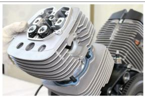
• Remove the cylinder head gasket
