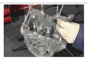
Insert the camshaft into the seat in the upper crankcase, lubricate and insert locking the camshaft locking fitting.
