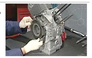
Tighten the screws and fit the specified flywheel locking tool.
