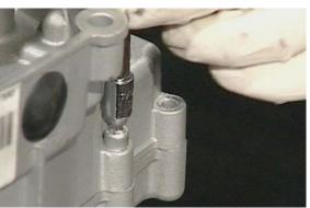
Detach and remove the clutch bell together with the clutch shaft tapping lightly around clutch bell edge.
