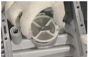
• Check that the mesh filter is not dirty, wash and blow with compressed air if needed.
