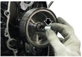
Place and tighten the tool (1) on the rotor.
