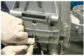
Insert the gear with its washer onto the gearbox primary shaft, tighten the retaining nut to the prescribed torque and squash with a punch.
