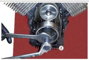
Operating on the alternator cover, proceed with the removal of the stator wiring lock plate
