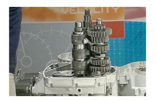
Slide off the pre-selector and remove the pre-selector seal ring.
