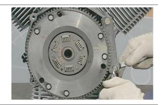
Unscrew the clutch plate fixing screws and remove clutch plate together with starting sprocket.
