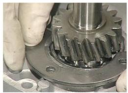
Undo the clutch shaft fixing nut.
