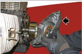
• Remove the rotor fixing screw
