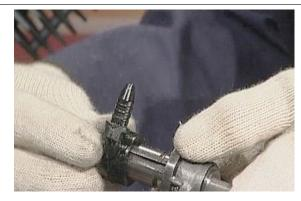
Insert the oil delivery fitting and the rockers on the shaft and lock them in place with the circlips.
