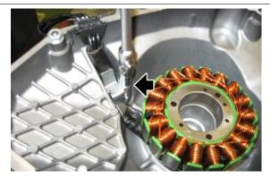
• Fix the stator with the three screws.
