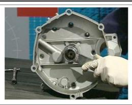
Slide off the clutch shaft and remove the seal ring.
