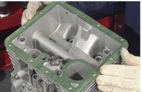
Tighten the sump screws following a crisscross pattern to the prescribed torque using a torque wrench.
