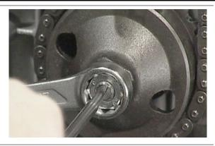
Fit the chain tensioner and tighten to the prescribed torque using a torque wrench.
