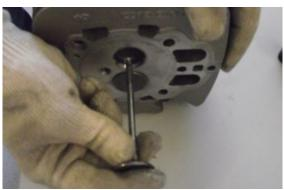
Remove the valve guide seals and extract the lower cap of the springs.
