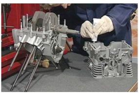
Join the two crankcase halves and tap lightly with a mallet to ensure that the two mating faces adhere together firmly; tighten the four central stud bolts and the external nuts following a crisscross pattern.
