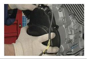
Unscrew the screws fixing the stator to the timing system cover and slide off the stator.
