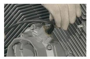
Position the engine speed sensor on the timing system cover and tighten the two fastening screws to the prescribed torque.
