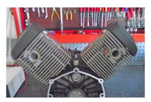
Tighten the screws following a crisscross pattern with a torque wrench set to the prescribed torque.
