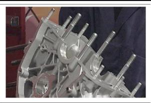
Blow all oil galleries of the two crankcase halves with compressed air.
