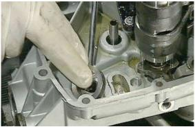
After unscrewing the retaining plate fixing screws, remove the complete set of gears, shafts and forks.
