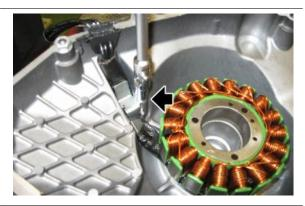
Removing the three stator fixing screws makes it possible to disconnect it
