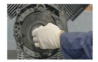
Unscrew the screws securing the pressure plate flywheel to the crankshaft and then remove it.
