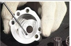
External rotor seat thickness 15.030 15.070 mm (0.5917 - 0.5933 in).
