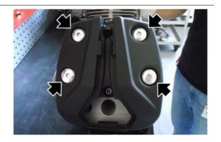
Loosen the central fastening screws
