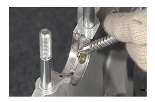
Insert the seal ring (after lubricating it)
