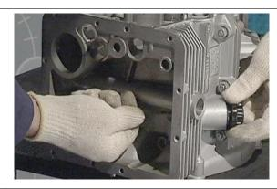
Straighten the safety plate, remove the mesh filter retaining screw from the oil sump and remove the mesh filter.
