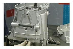
Unscrew the gearbox cover bolts and remove the cover tapping it with a mallet.
