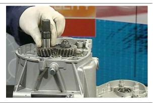
Install the specified locking tool onto the clutch shaft splines.
