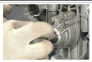
Fit the two gears with the timing chain; after installation, check the position of the reference notches and tighten the screws to the prescribed torque with a torque wrench.
