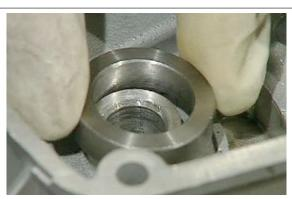
Fit the selector onto the cover making sure that the two tangs of the spring locate into the adjuster screw groove, then turn the screw by 90° and tighten the lock nut.
