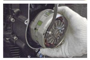
Unscrew the nut fixing the rotor to the crankshaft, slide off the rotor, remove the key and collect the washer.
