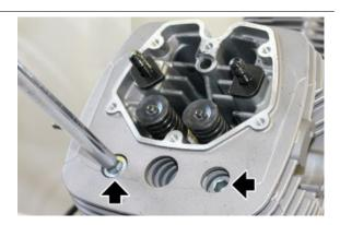
Remove the complete head from the cylinder
