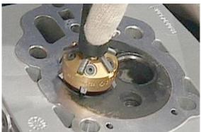
Repeat the procedure using the suitable cutter to achieve the correct valve seat sealing surface.
