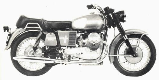
Engine: twin cylinder, 4-stroke - Compression ratio: 9.2 to 1 - Output: 64.5 HP at 6500 r.p.m. - Starting: electric - Clutch: twin dry discs - Gearbox: 5 speeds, foot operated -Transmissions: primary by gears, secondary transmissions: primary by gears, secondary by cardan shaft - Suspension: telehydraulic - Brakes: central hub - Tyres: 4.00 x 18 - Fuel consumption: 6.5 l. x 100 kms. (43 m.p. g. imp.) - Weight: 230 kgs. (506 lbs.) - Top speed: over 190 kms/h (119 m.p.h., w/o windshield).
