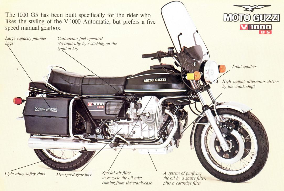
The 1000 G5 is equipped with the integral braking system, patented by Moto Guzzi in 1975. This major contribution to motorcycle safety won presented by the German Automobile Club and is acknowledged as the safest motorcycle braking system by specialised press all over the world.
