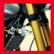
The V11 Cafè Sport is fitted as standard with an Öhlins fork with solid 43 mm inners and distinctive gilding. Thanks to Its particular characteristics, the bike enters bends with precision and follows an ideal trajectory on the straight. The damper on the sensitive and responsive steering also bears the Öhlins signature.
