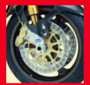
Extreme braking performance and powerful progressive stopping, thanks to the powerful double 320 mm diameter front disc brake, operated by a Brembo caliper with four opposed pistons. A system which adapts perfectly to different riding styles, always offering maximum safety.
