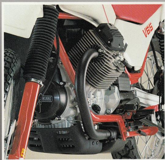
MOTORE BICILINDRICO A V90° CON I CILINDRI BEN ESPOSTI AL RAFFREDDAMENTO
