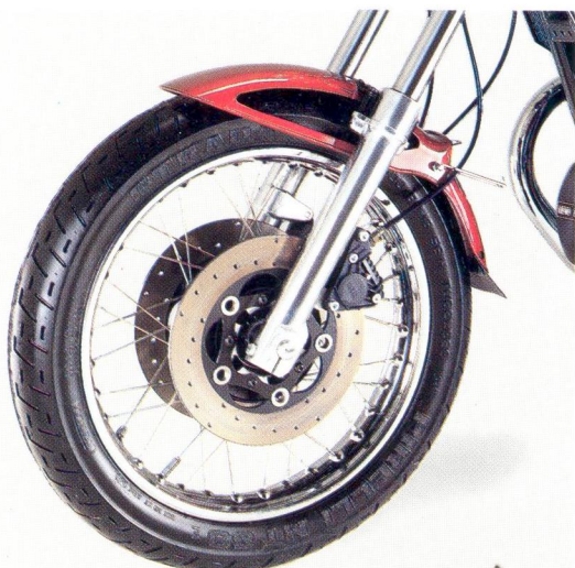
FRONT DOUBLE FLOATING DISC BRAKES FOR 750 NEVADA ONLY
