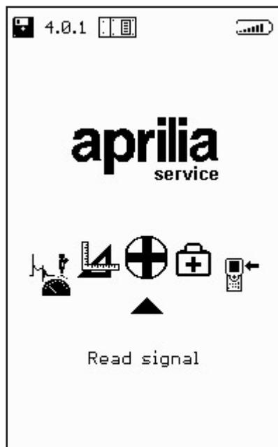
The AUTO-DIAGNOSTICS program is used to connect the AXONE2000 APRILIA to various injection ECUs with different characteristics according to the make and the specific injection system.
