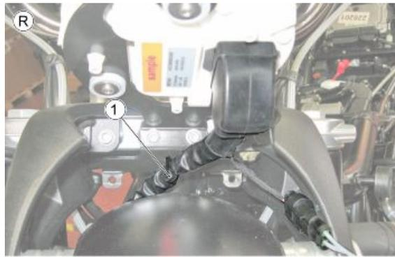
**TAFEL S - EINBAU LUFTTEMPERATURSENSOR**
