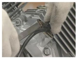
• Remove the washer, smear the plate with suitable sealant, fit the sensor and tighten the screws to the specified torque.
