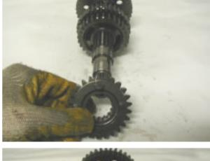
Remove the circlip.
