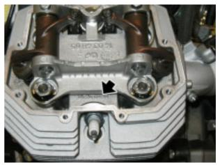
• Change the gasket and install the head cover, see REMOVING THE HEAD COVERS.
