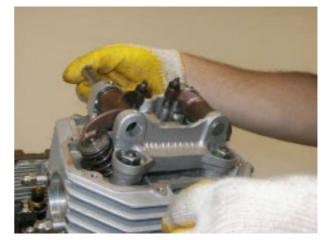
• Remove the rocker arm shafts.
