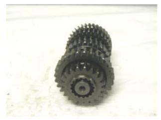
• Remove the second speed gear, set aside the roller cage.
