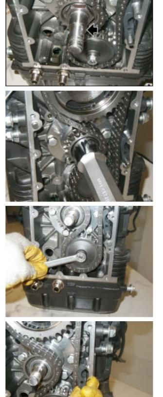
• Slide out the pick-up ring and set aside the dowel.
