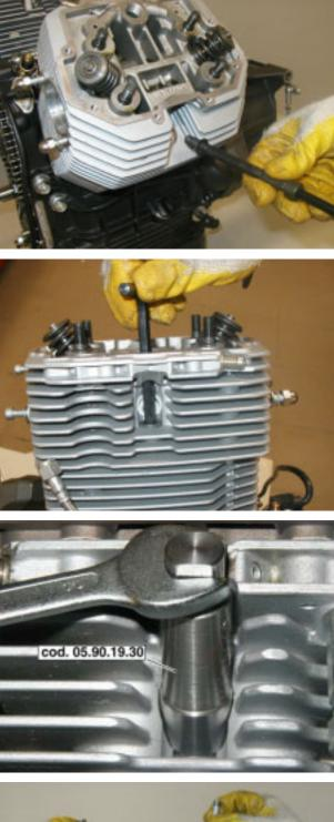
• Using the suitable special tool (part no. 05.90.19.30), tighten the internal spark plug.
