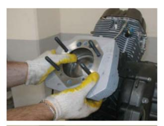
• Fit the gasket at the cylinder base.
