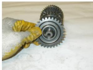
• Remove the circlip.
