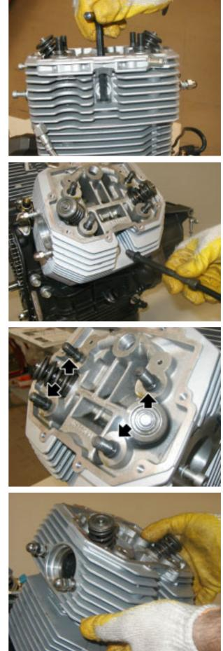
Slightly detach the head from the cylinder and remove the four O-rings.
