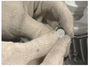
• Position the sensor on the timing cover and place it against the pick-up ring.
