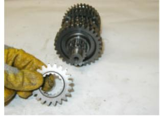
• Remove the sixth speed gear and set aside the washer.
