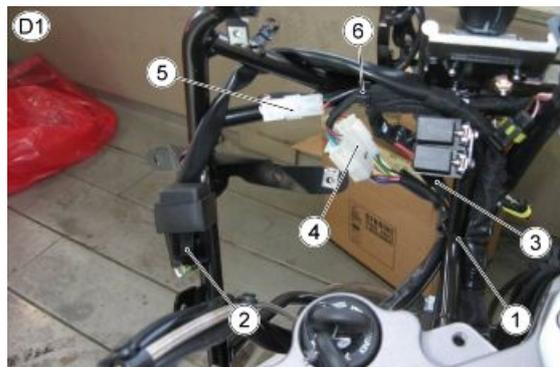
**FRONT SECTION - TABLE D2: FRONT MAIN CABLE HARNESS**
