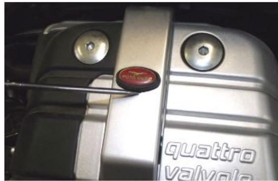
If the timing system is very noisy, check the clearance between the valves and the rocking levers.
