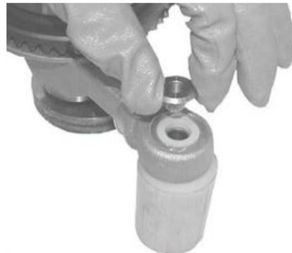
Remove the sealing rings (2) and (7) with a screwdriver.
