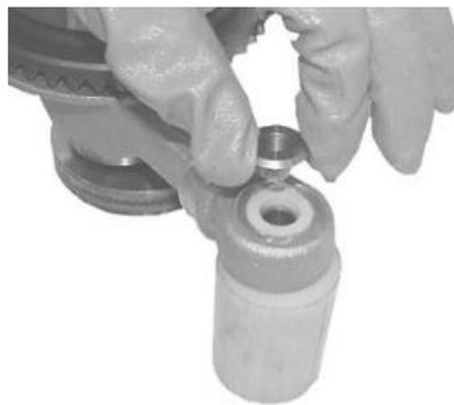
Drive the bushing (1) in with a plastic hammer.
