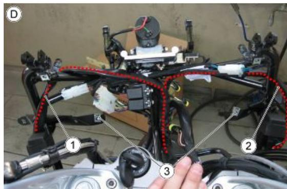
**FRONT SECTION - TABLE D1: FRONT MAIN CABLE HARNESS**
