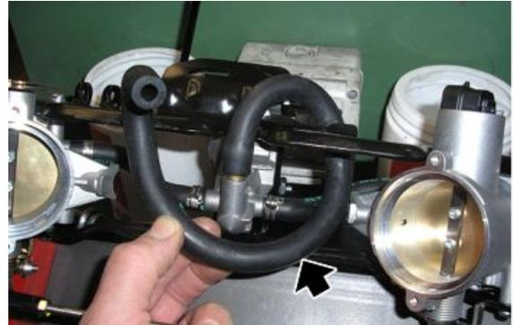
The shortest part of the fuel pipe connected to the throttle bodies should be placed on the right.
