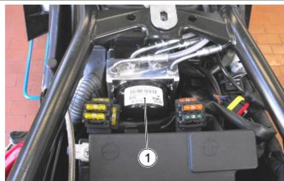
When sensors (3) detect a significant speed difference between the rear and the front wheels (for example, when rearing up on the back wheel), the ABS system could take this as a dangerous situation. In this case, 2 things may occur:
