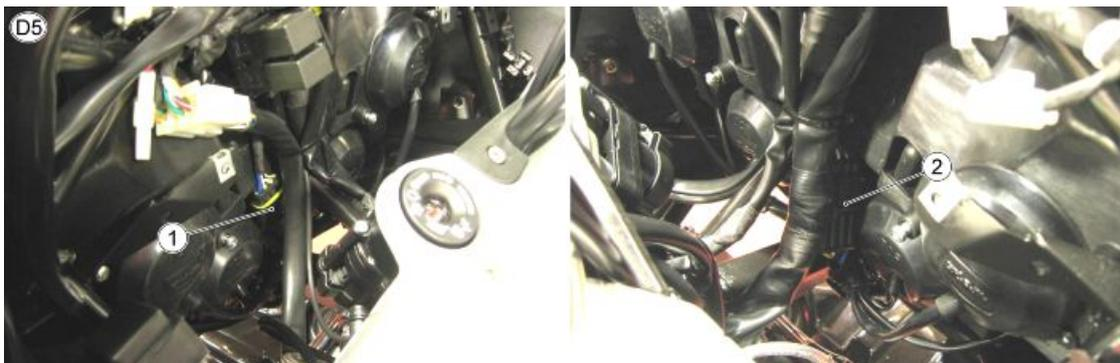
**FRONT SECTION - TABLE E: FRONT ABS SENSOR**
